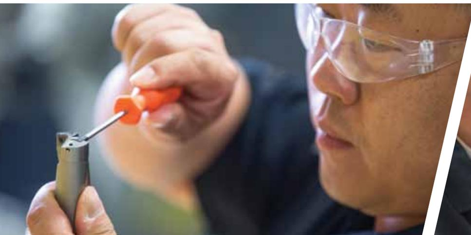
*An engineer is securing the drilling insert to a prototype of WIDIA's new Top Cut Four indexable drilling platform.*
