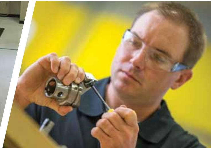
*A technician is working to ensure that the KM4X63 cutting unit prototype is built precisely to design specifications for a Top Notch Insert.*
